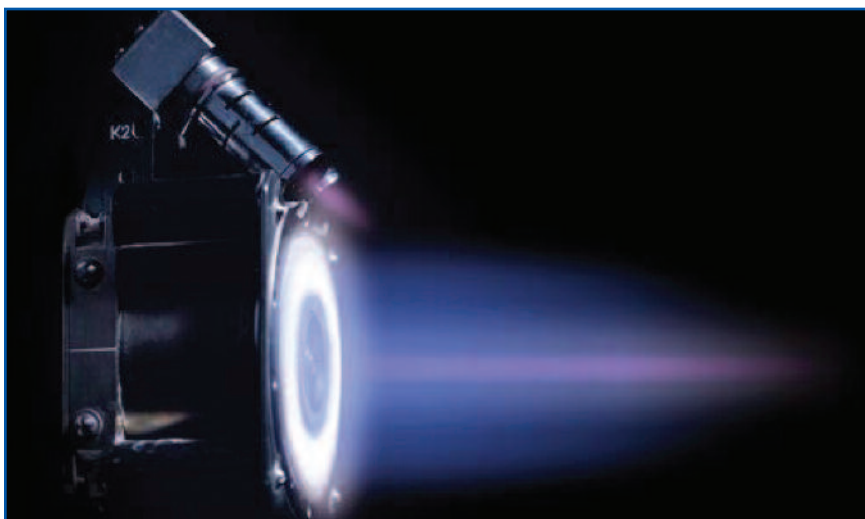
Figure 2b. Plasma flow coming from the closed drift ion source of magnetic layer type SPT-100. Hollow Cathode neutralizer is on the top.
